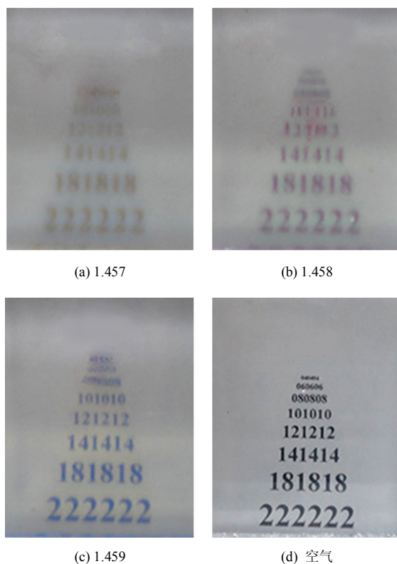
图 1 在 21℃ 下孔隙溶液折射率对透明土透明性的影响 Fig.1 Effect of refractive ratios of pore fluid on transparency of transparent soil at 21℃
